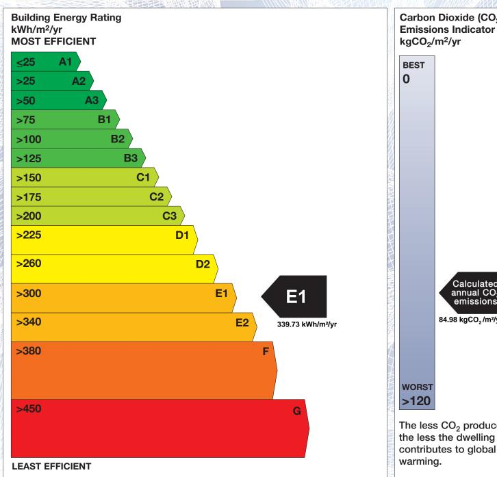
Carbon Dioxide (CO<sub>2</sub>) **Emissions Indicator** Calculated annual CO2 emissions 84.98 kgCO<sub>2</sub>/m<sup>2</sup>/yr The less CO<sub>2</sub> produced,
